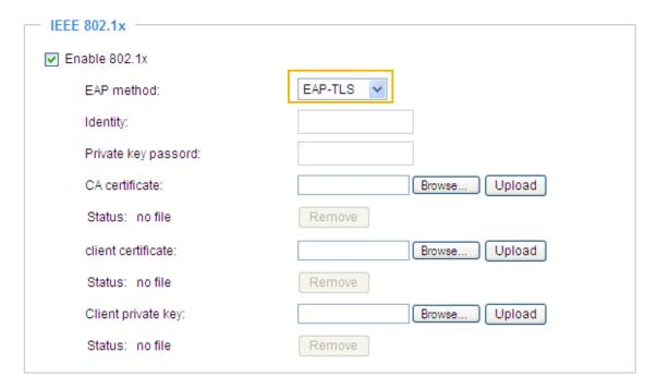
3. When all settings are complete, move the video server to the protected LAN by connecting it to an 802.1x enabled switch. The devices will then start the authentication automatically.
